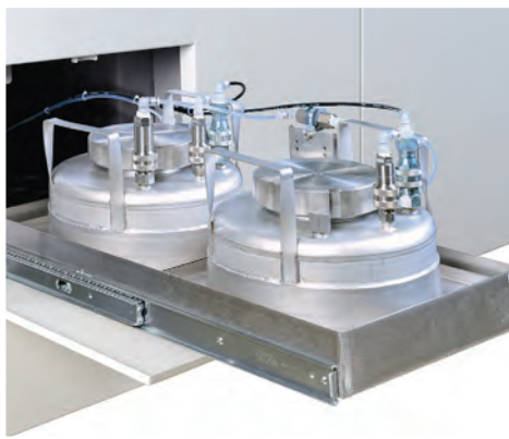
Flux and solder can be added without stopping manufacturing
